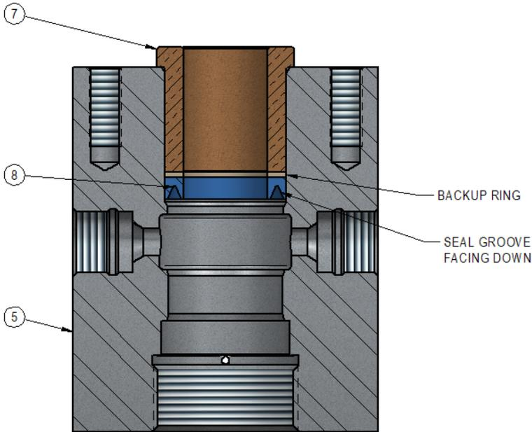
2. Install the o-ring (Item 3) and backup ring (Item 9) onto the seat (Item 17). The ID chamfer on the backup ring should be on the side opposite the o-ring. Apply o-ring lube to the o-ring.
