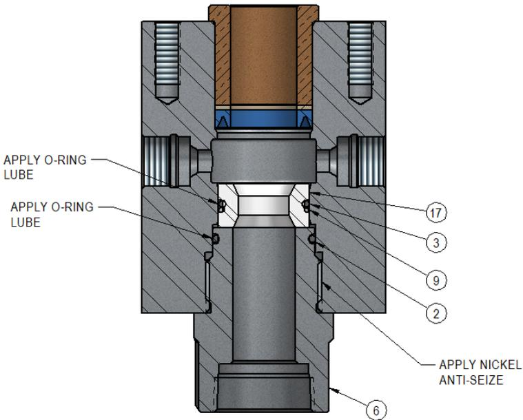
5. Install the valve plunger (Item 13) by pushing it through the guide bushing (Item 7) and seal (Item 8) until it contacts the seat (Item 17).
