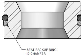
3. Install the seat (Item 17) into the body (Item 5) with the o-ring on the side closest to the center of the body as shown. The seat does not need to be pushed down into its final position in this step, but it should be centered in the body to prepare it to be pushed into position.
