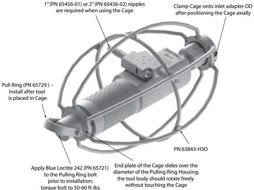
**NOTE:** Only 1" or 2" extensions can be used when the H<sub>3</sub>Orbiter is installed in the centralizer. Pull ring and Inlet adapter required to secure the H<sub>3</sub>Orbiter in the cage.
