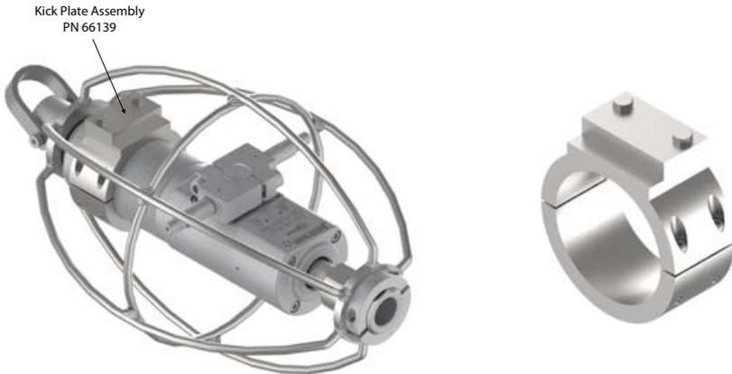
**NOTE:** Effectiveness of the kick plate is dependent on tool setup (nozzle/manifold) and material in pipe. At 20K operation, a minimum flow of 17 gpm with the R90 manifold is recommended. Use of the R150 manifold with the kick plate assembly is not recommended.
