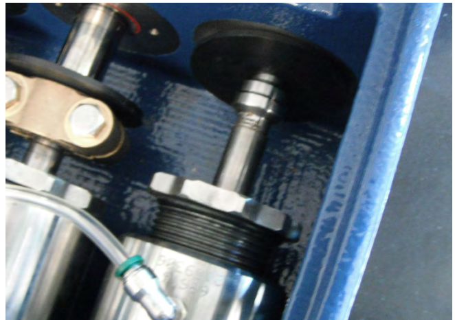
Figure 69: Pull Plunger to Meet Pony Rod.
