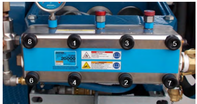
Figure 30: Bolt Tightening Sequence.
