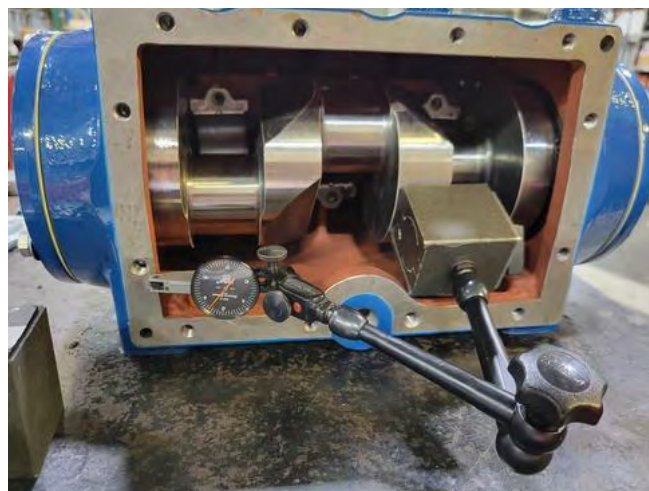
Figure 142: Mount Magnetic Base Dial Indicator
