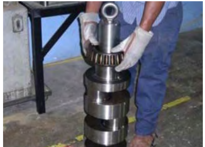
Figure 168: Place Heated Bearing
