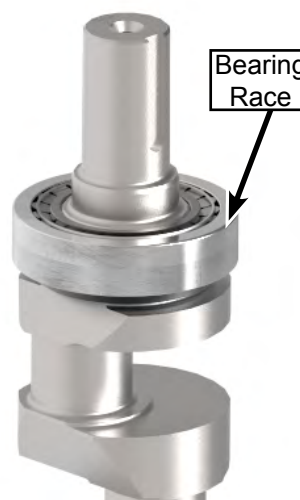
Figure 135: Install the Outer Bearing Race.
