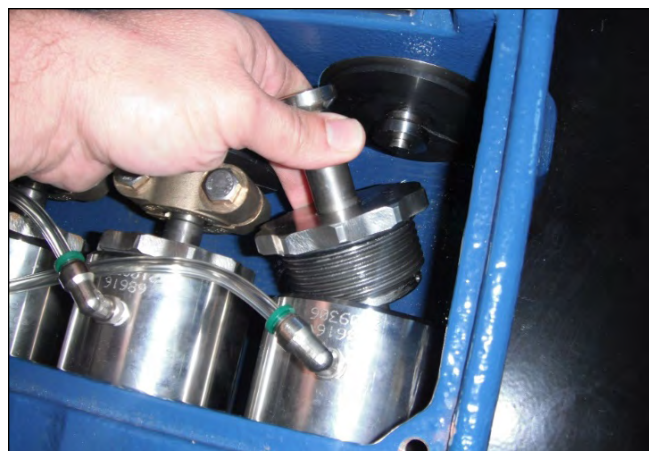
Figure 65: Remove Gland Nut and Plunger Assembly.
