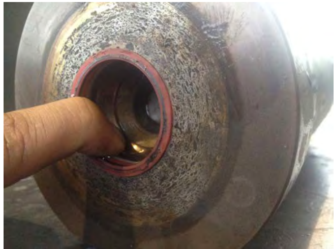
Figure 76: Gently Remove 40K Face Seal from Stuffing Box.
