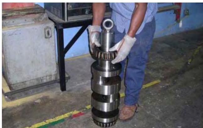
Figure 151: Install the Heated Bearing Using Proper PPE
