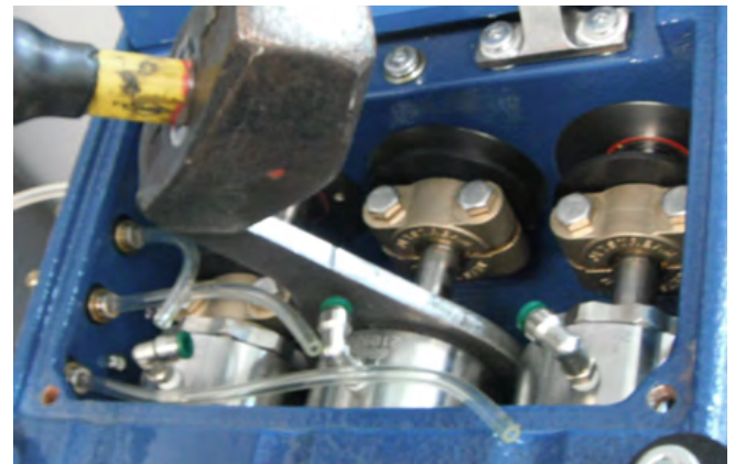
Figure 46: Tightening Gland Nuts.
