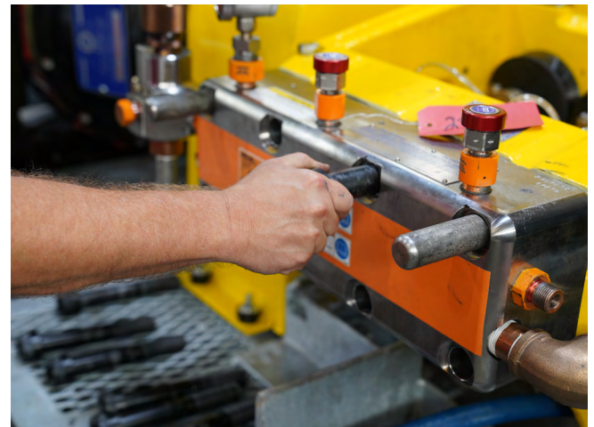
Figure 73: Install Manifold Studs.
