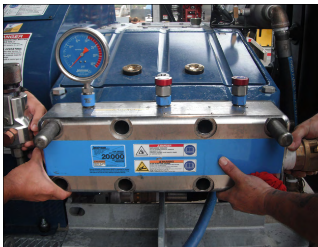
Figure 25: Install the New Manifold.
