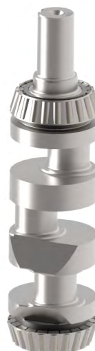
Figure 134: Slide Hot Bearings onto Vertical Crankshaft.
