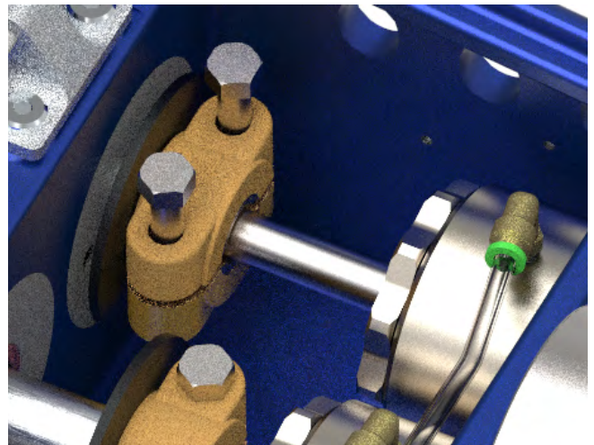
Figure 70: Install Plunger Coupling.
