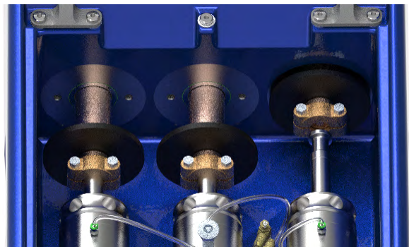
Figure 163: Remove Plunger Couplings
