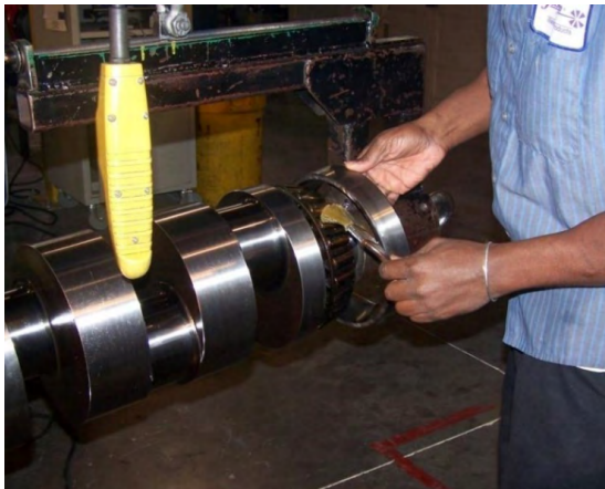
Figure 174: Apply Oil to Bearings
