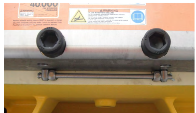
Figure 74: Check Trunnion Rod Before Lowering Manifold.
