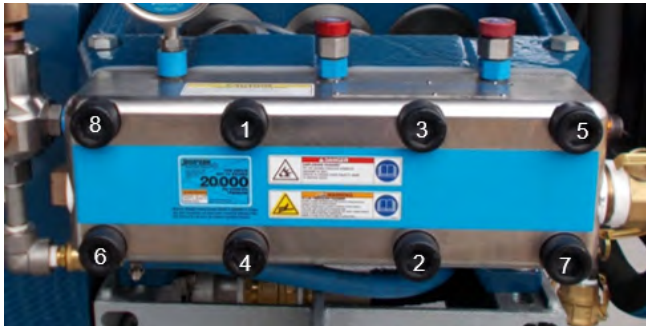
Figure 78: Manifold Bolt Tightening Sequences.
