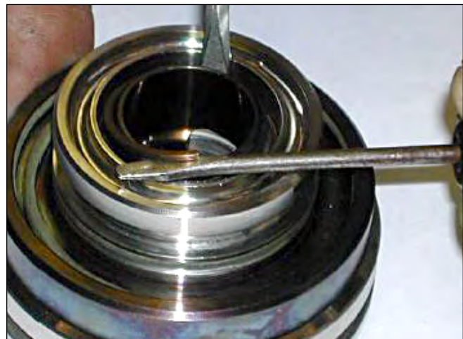
Figure 81: Remove Spring Retainer.
