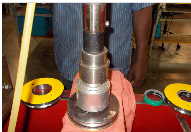
Figure 112: Install Inboard Seal.
