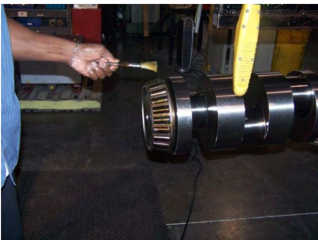
Figure 157: Apply Oil to Bearings
