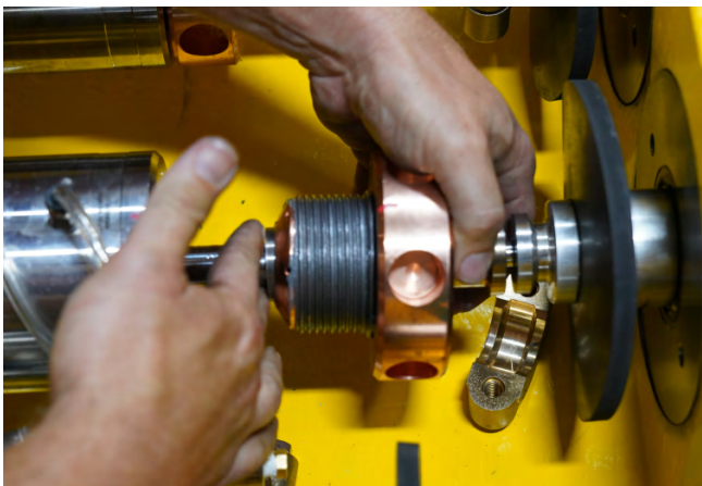
Figure 59: Reinstall the Plunger Assembly into Stuffing Box.
