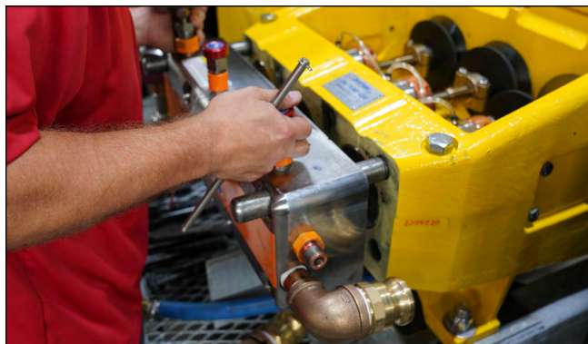
Figure 26: Manifold in Adjustment Position.
