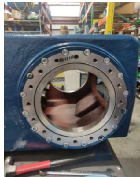
Figure 170: Install Outer Race in Power Frame
