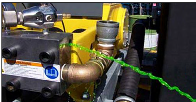
Figure 14: Draining the Anti-Freeze.
