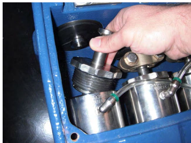
Figure 68: Install Gland Nut and Plunger Assembly.
