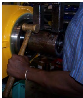
Figure 158: Tap in the Bearing Race
