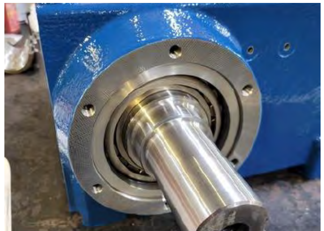
Figure 140: Install Side Bearing Race.
