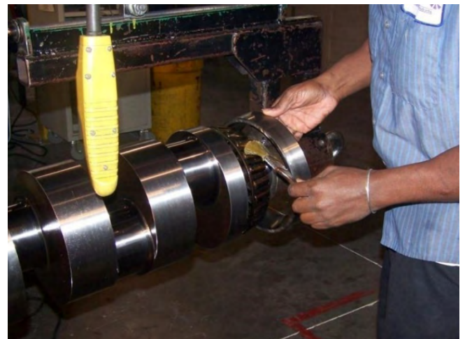
Figure 157: Apply Oil to Bearings
