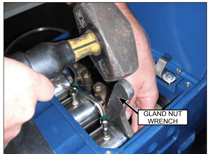
Figure 63: Remove Gland Nuts.
