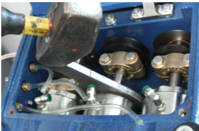
Figure 23a: 2000 Pump Gland Nut Installation
