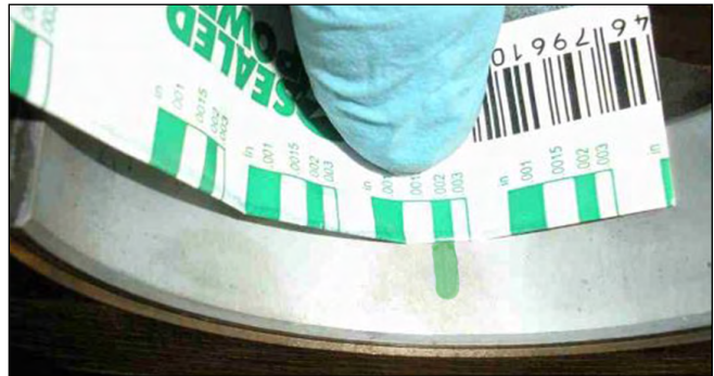
Figure 119: Measure Flattened Plasti-Gauge.
