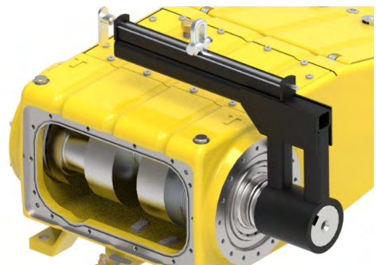
Figure 148: Install Lifting Tool
