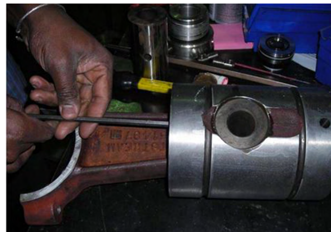
Figure 129: Second Set Screw Installation.
