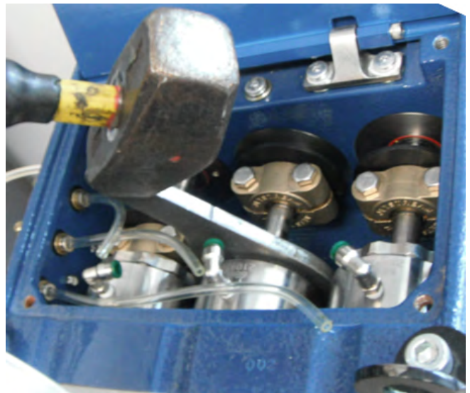
Figure 71: Tighten Gland Nut.
