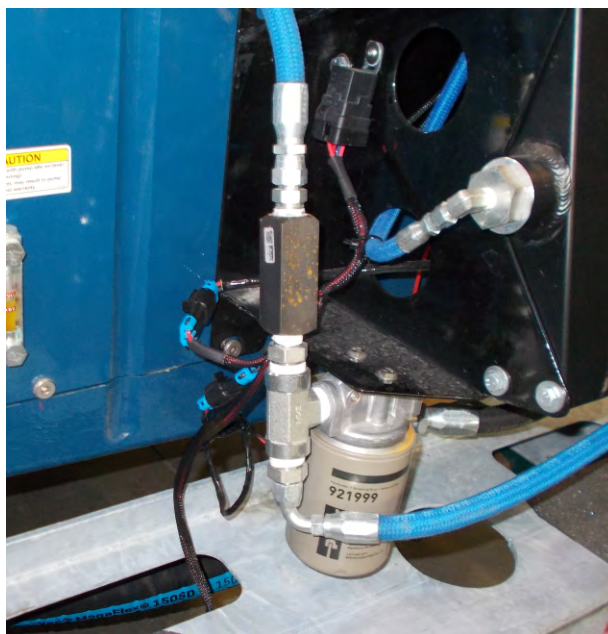
12/24V Field wiring to pump harness
