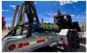
NEW AND ENHANCED FEATURES: Reduced deck height provides easier access to pump components while performing routine maintenance. Plus, geared jack stands for more efficient adjustment and leveling and upgraded rigid hard pipe connections.
